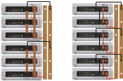
Figure 5-1 Schematic diagram of power cable connection
